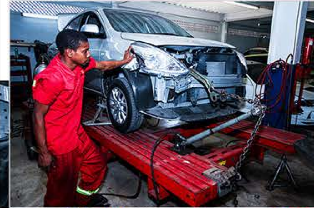
< 5 Chassis Repair Machines
